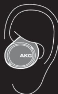
Turn the earpieces backwards when slotted in your ears to find the most optimal wear position for advanced touch controls - the AKG logo should be horizontal when worn.
